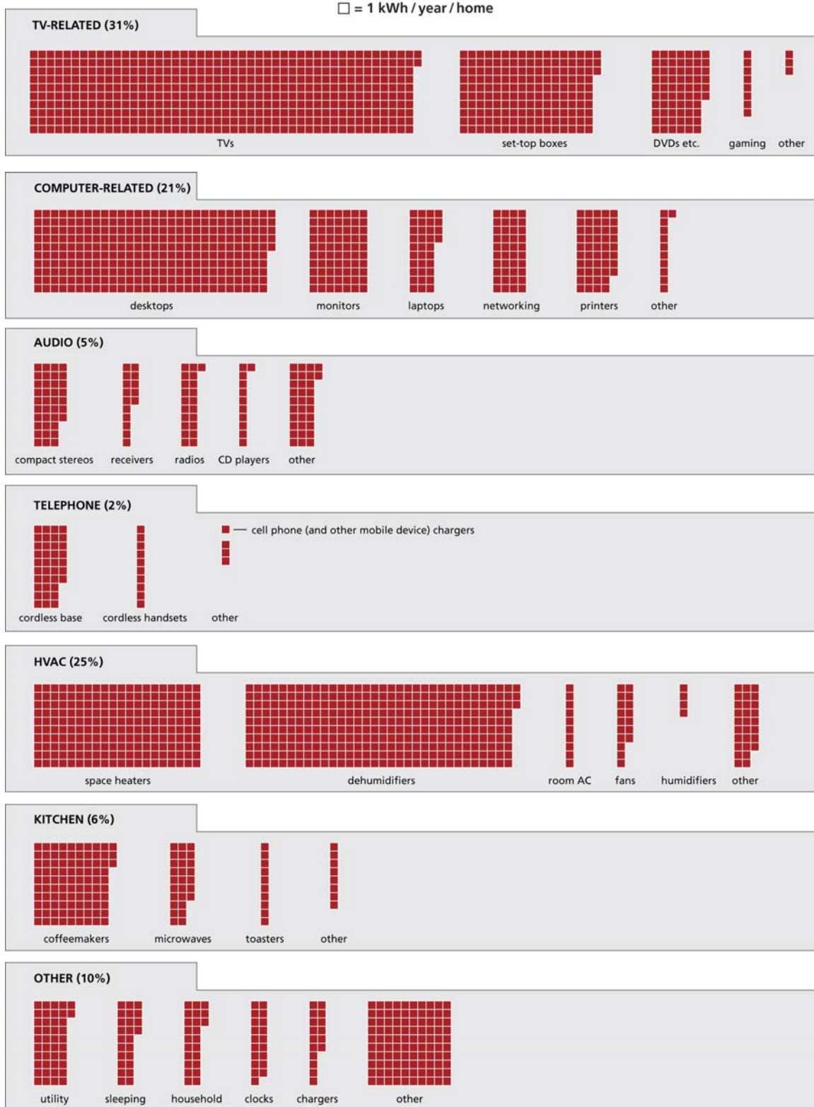
Figure 1. Point estimates of electricity use for miscellaneous plug-in devices in Minnesota single-family homes (2,300 kWh/year/home)
